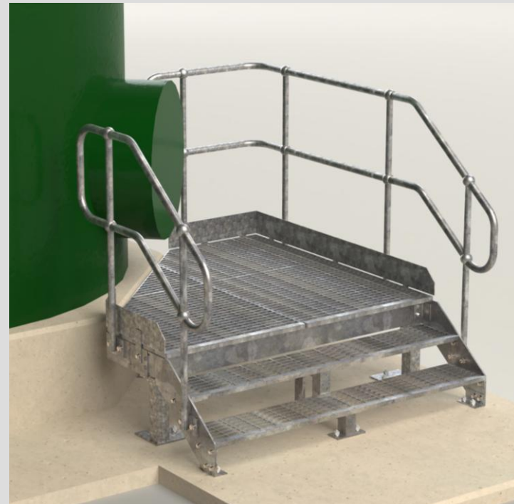
Above – Finished installation of 1855x1670x53mm Access Platform. With Staircase and Handrailing.
